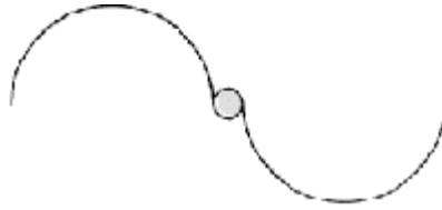
This is the design I use. it is very strong due to the central shaft, but slightly less efficient than the other two. However, the extra strength allows the rotor to be supported at one end only.
