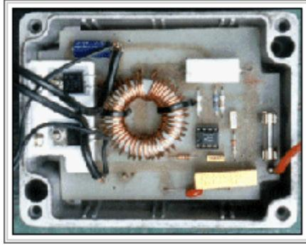
The step up converter built from a kit. It starts from just four volts and outputs a regulated 14 volts to the battery
