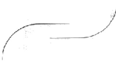
This is the most efficient Savonius design. It not only has the advantage of air being deflected twice like the design above, but also that the vanes act partly like an airfoil when they are edge-on into the wind, creating a small lift effect and thus enhancing efficiency. This design is much more difficult to build, requiring vanes rolled from metal sheet instead of being cut from drums or pipes.
