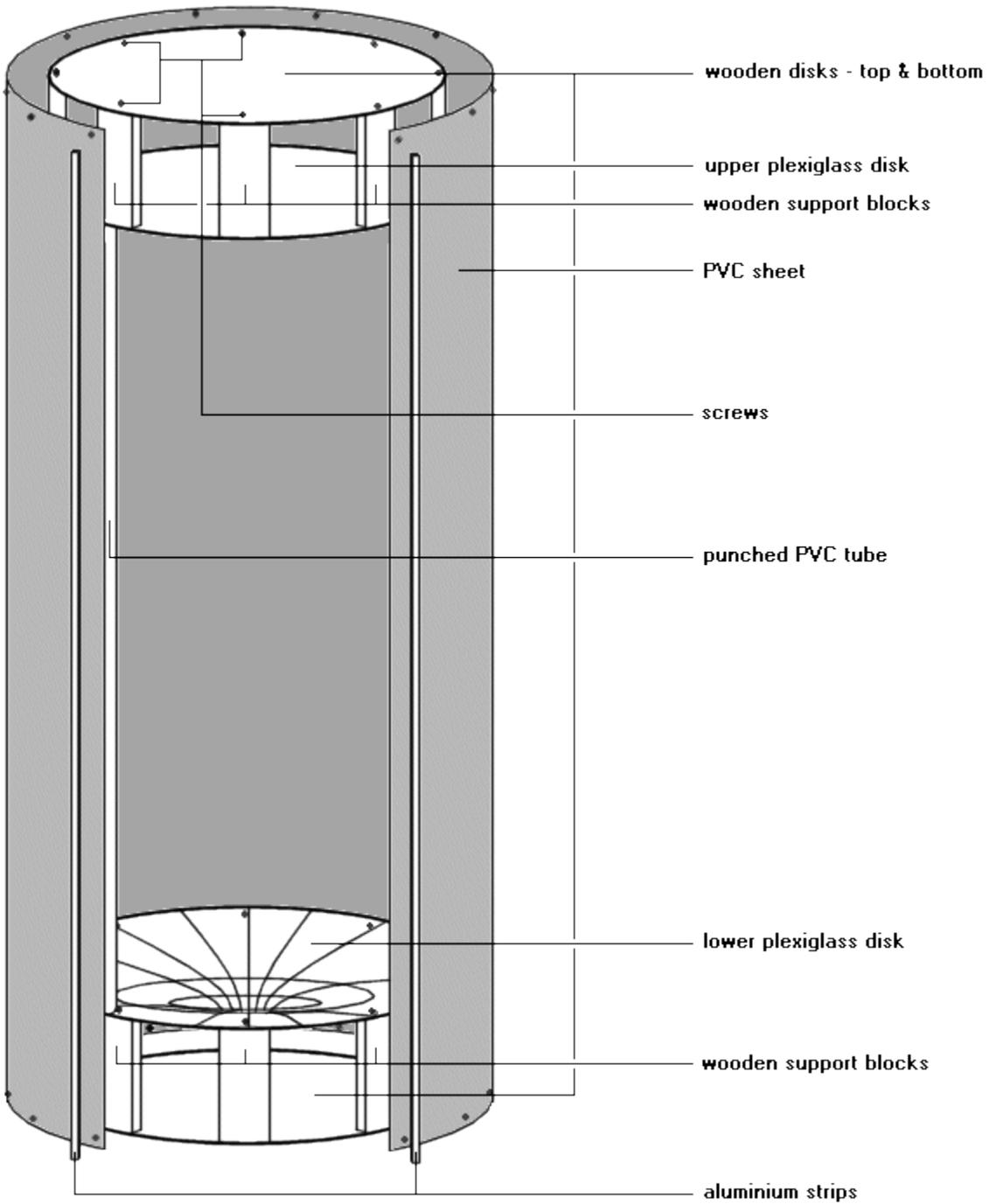
Cutting the wooden disks and support blocks
