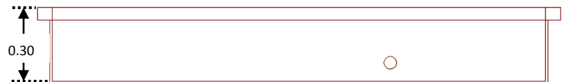
Figure 29: Side view of grow bed with dimensions in meters (not to scale)
